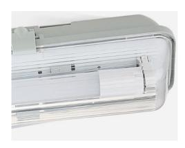
The LEDVANCE® DampProof Housing is an IP65 empty housing designed to work with IEC 62776 compliant LED T8 tubes with AC input on one end. Its fused design offers additional protection when inserting traditional T8 florescent tubes by mistake. It is available in 3 lengths with 1 & 2 lamps versions to fulfill different applications requirements.
