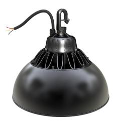
The LEDVANCE® Value Highbay is a high efficient and reliable LED luminaire, designed for industry and commercial applications. Smooth and beautiful line of the shape of housing. Unique heat dissipation design: air convection hole made, both Alu reflector and plastics heat sink dissipate the heat together. Anodized aluminium reflector help to control glare. It is the perfect solution for one to one replacement of HID conventional luminaire.
